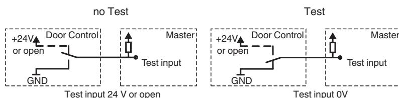
If the device is not used as a safety sensor in accordance with DIN 18650 / EN 16005, there is no need to connect the test input.
